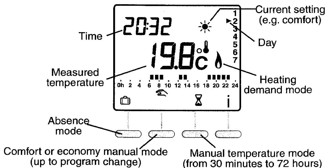
When starting up, the temperature measured by the thermostat is displayed (the **°C** symbol appears above the **°C**).
