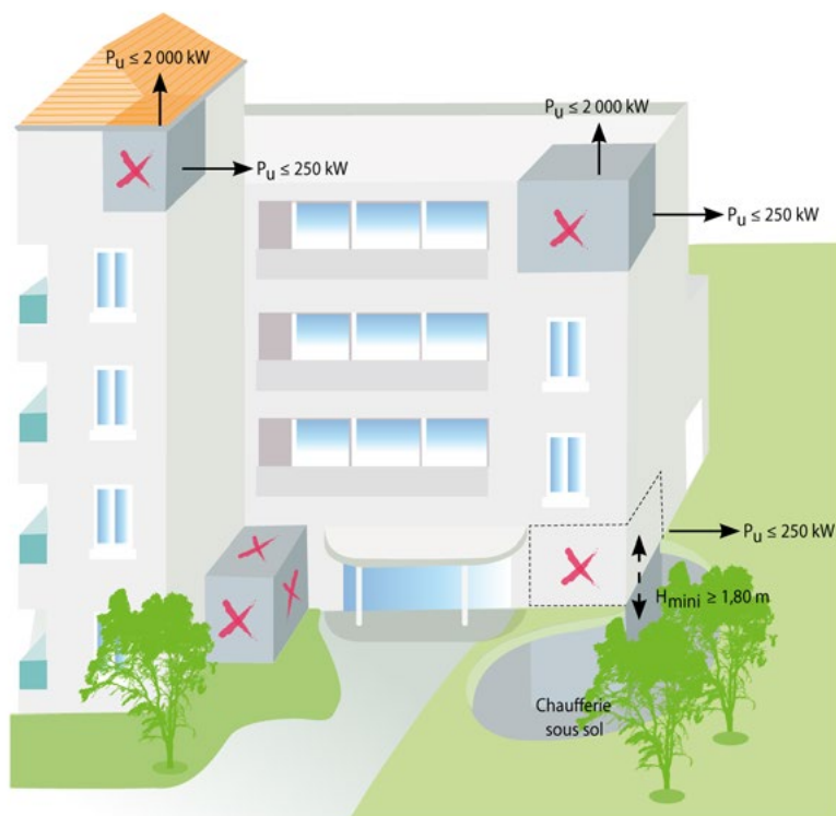
figure 7 - Implantation terminaux ventouse (suite)
